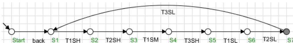
Fig. 31. Auxiliary automaton C for Tr_{02.2} .
